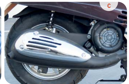
Features Shown: A - Headlight. B - Speedometer. C - Chrome Muffler Shield.
