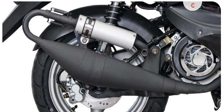
Features Shown: A - Aerodynamic Windshield. B - Taillight. C - Rear Disc Brake & Sport Muffler.
