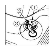
3 LOCK position Turn the switch all the way to the left, push it down and turn it to the LOCK position; the key can be pulled out. In this case, the vehicle can not be steered and the engine as well as the lighting system will not work.
