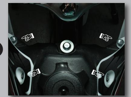
Remove four screws that hold the front of the bike's seat to the fuel tank
