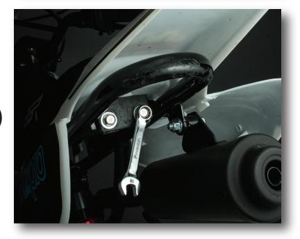
Uninstall the seat by removing the two screws underneath and slide back.
