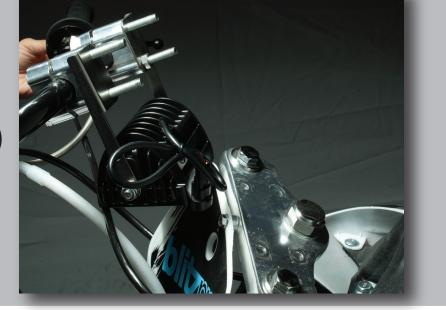
Install the headlight with brackets by lining it up with the four stem bolts
