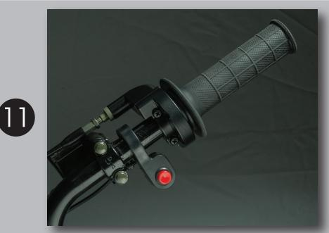
Install switch by removing throttle grip with a Phillips screw driver. Slide switch onto bar and tighten with 2.5mm hex key.
