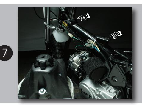
Remove the two screws holding the fuel tank. Cut ziptie to access the wires.
