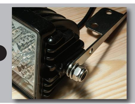
Begin first by installing the brackets onto the light with the tabs pointing inwards
